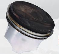
The piston crown contains normal carbon, while the rings remain clean and functional. Note the absence of wear or scuffing on the piston skirt. The camshaft shows little-to-no scoring, bluing or wear after 3,000 miles of high-performance racing.
